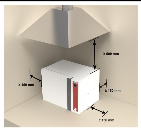
Depending on the application of the product, it may be appropriate to position it under an extraction hood. Ensure the extraction hood is switched on during use.
